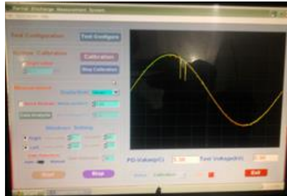
Fig 7: Partial Discharge test result in new manufactured 185 sq. mm cable drum tested.
